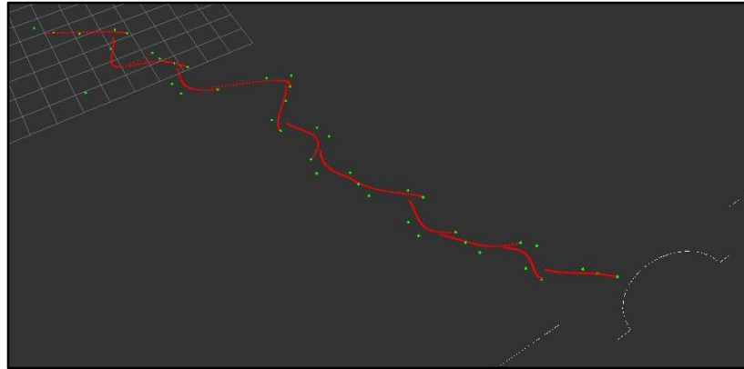
Figure 13: 6-point Bezier curve (Green points are guidance points & red are Bezier Points)
